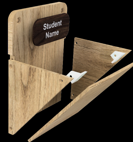
Figure 4 - Exploded view of the unit, showing how it will be assembled and attached to the frame
